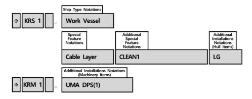
Remark: In relation to Special Feature Notation, A\*(Purpose), Offshore Support Vessel's special feature notations, FFS1, FFS2, FFS3 or FF, shall be assigned to ships if they are complied with Ch 8 of Guidance for OSV and the requirements of FFS1, FFS2, FFS3 or FF, which are Special Feature Notations of Offshore Support Vessel.
