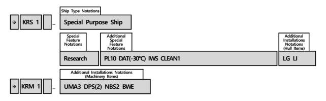
Remark: In relation to Special Feature Notation, A\*(Purpose), Offshore Support Vessel's special feature notations, FFS1, FFS2, FFS3 or FF, shall be assigned to ships if they are complied with Ch 8 of Guidance for OSV and the requirements of FFS1, FFS2, FFS3 or FF, which are Special Feature Notations of Offshore Support Vessel.
