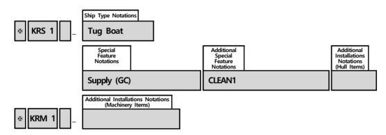
Remark: In relation to Special Feature Notation, A\*(Purpose), Offshore Support Vessel's special feature notations, FFS1, FFS2, FFS3 or FF, shall be assigned to ships if they are complied with Ch 8 of Guidance for OSV and the requirements of FFS1, FFS2, FFS3 or FF, which are Special Feature Notations of Offshore Support Vessel.
